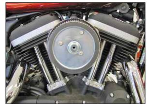
10. Install the K&N<sup>®</sup> air filter onto the back plate and secure with the provided hardware. **NOTE: Be sure to place one drop of the provided thread locker onto the threads of the bolts.**
