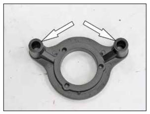
6. Install two of the provided O-Rings into the K&N<sup>®</sup> throttle body bracket as shown.
