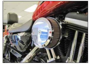
11. Install the filter cover and secure with the provided bolt.
