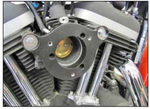
7. Install the two remaining O-Rings into the front side of the K&N<sup>®</sup> throttle body bracket, then insert the two provided breather bolts through and attach the assembly to the cylinder heads but do not completely tighten. Insert the provided throttle body gasket and then install the filter spacer bolts to hold the gasket in place. Tighten the breather bolts and then remove the filter spacer bolts.
